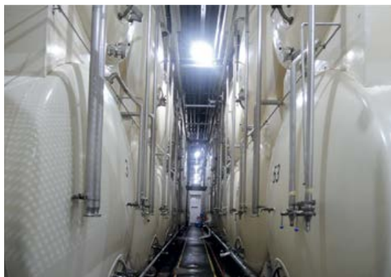
Level sensors in beer tanks monitor level and fill and can be networked to the brewery's order and supply systems.
