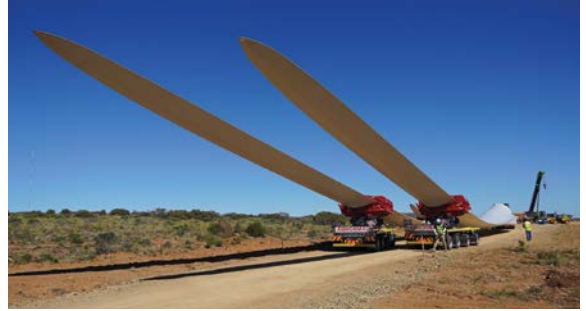
The turbine blades for Koruson 1, each 81.35 m long and weighing 28 tonnes, in transit to the site.
