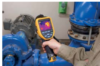
Thermal imaging cameras can be used to monitor plant and equipment and detect anomalies.
