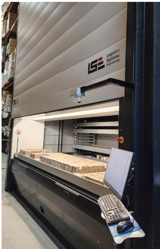
The new VLM delivers greater functionality and requires much less space than conventional racking and shelving.
