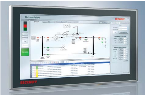
Operation and monitoring of the grid simulation at the Institute of Electrical Energy Systems and High Voltage Technology (IEH) at the Karlsruhe Institute of Technology (KIT) created with TwinCAT HMI.
