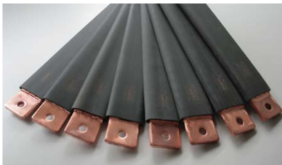
Cu-flex copper busbar is made of strands of copper wires woven into a flexible busbar with the ends forged into a solid unit.
