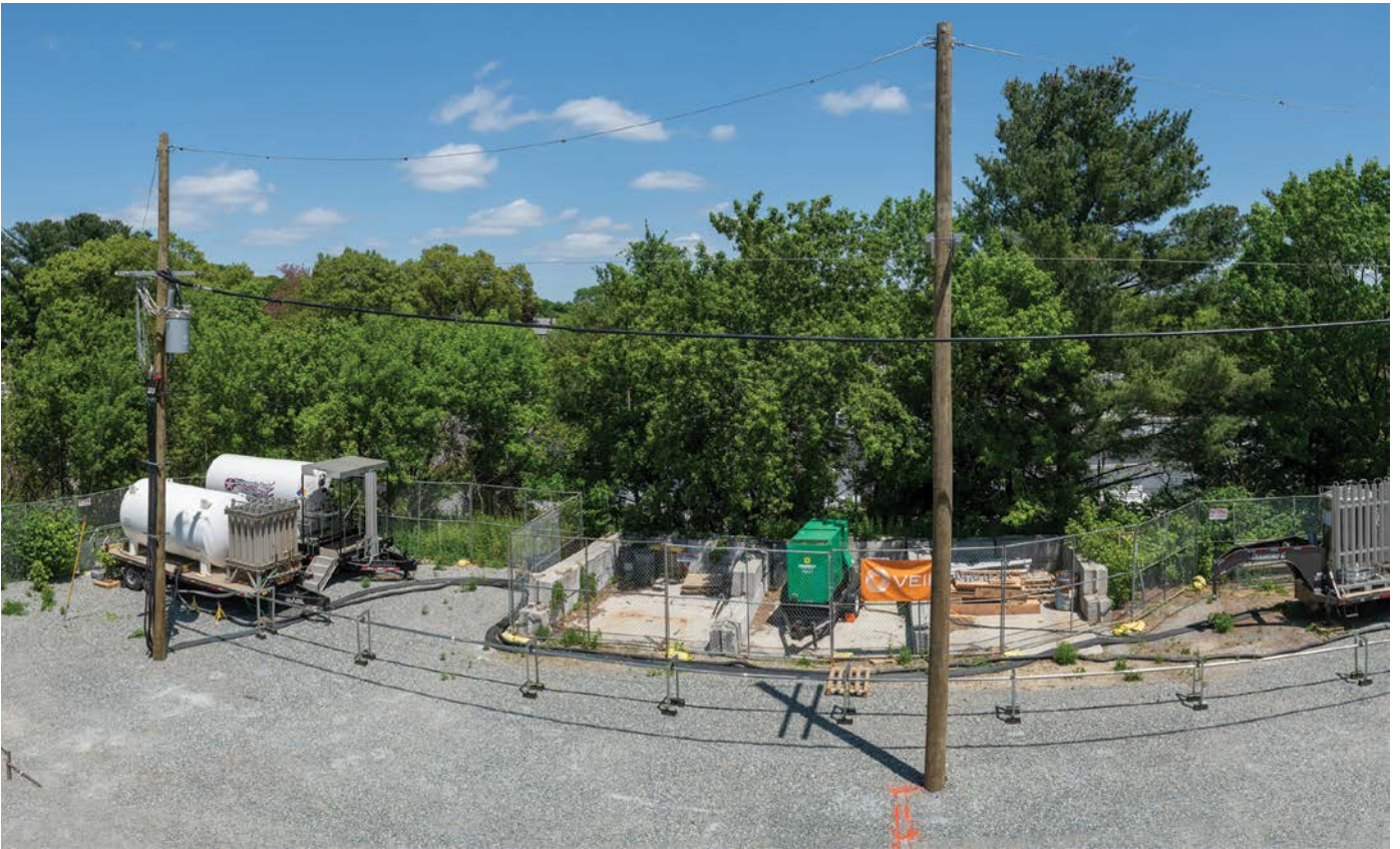
The core innovation at VEIR is the cooling system, which is passively cooled with nitrogen.
