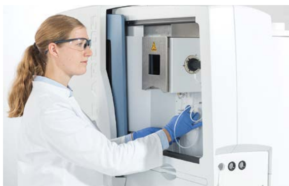
The SPECTRO ARCOS MultiView ICP-OES is used in analysing black mass from recycled lithium-ion batteries.
