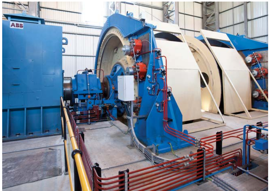
The mechanical, electrical control and drive systems for ABB mine hoists are fully designed in-house.
