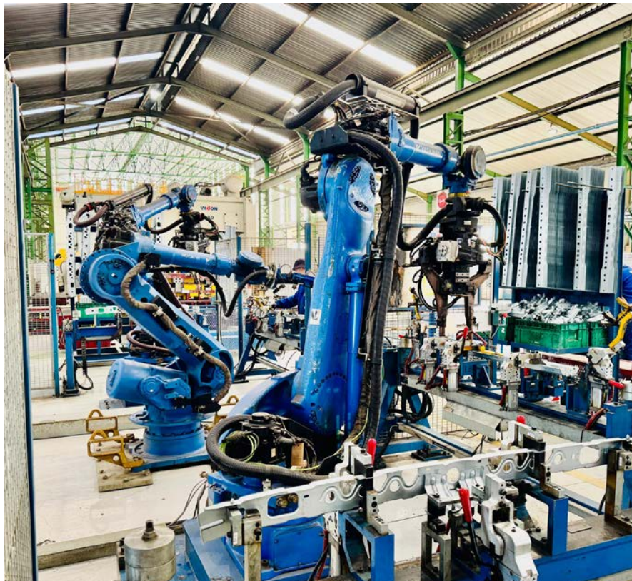
Malben Engineering makes use of automated robotic welding in its production of welded assemblies for the automotive sector.
