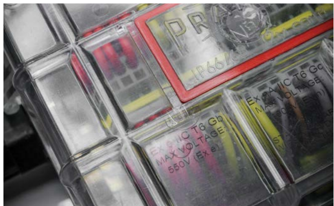
Rectangular Envirobox with polycarbonate lid, also showing the IP rating.
