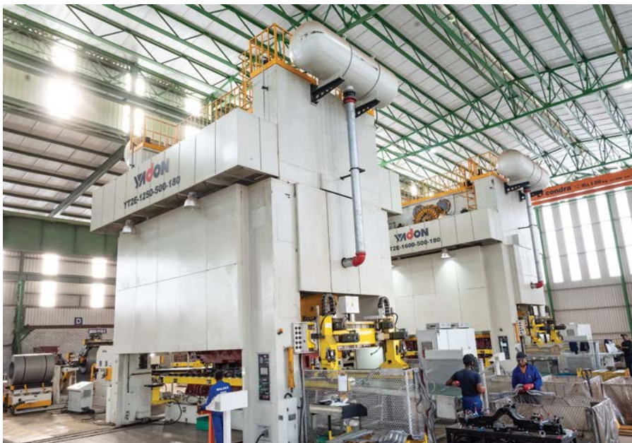
The Plant 2 press shop at Malben Engineering, showing 1 200- and 1 600-tonne Yadon presses.
