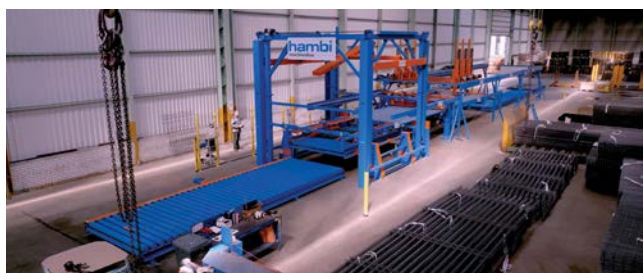
Hambi has developed a world-first system that automates the cutting, handling, and stacking of heavy reinforcing steel mesh.
