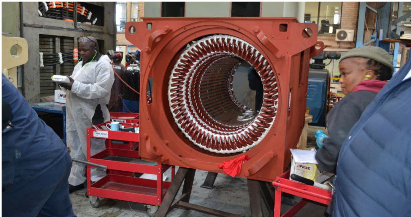
Form-wound copper stator coils being installed for a motor at Marthinusen & Coutts' Cleveland facility.
