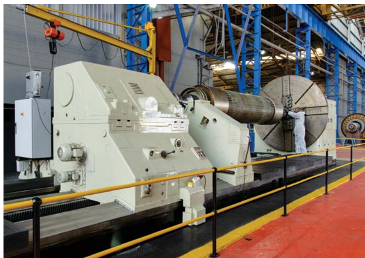
For very large machines, the Benoni facility includes a 140 t Wagner lathe that can accommodate a 40 t, 11 m workpiece with a swing of 3.2 m.
