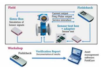
tors like FieldCheck from Endress+Hauser carry out the entire process automatically by controlling the flowmeter, simulating the measured values and documenting the results for further processing. Despite this, external verification is a very complex procedure that requires access to the measuring point in
