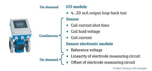
Tests that are part of the continuous self-monitoring are used for flowmeter diagnostics. They provide an immediate diagnostics event which allows it to react quickly and targeted to a device defect or an application problem.
