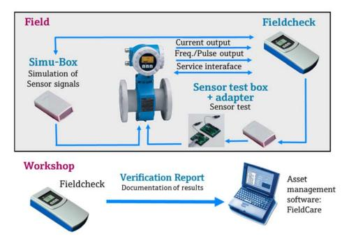
The status of verification and created data are subsequently used for documenting the results in a verification report. Modern verificators like FieldCheck from Endress+Hauser carry out the entire process automatically by controlling the flowmeter, simulating the measured values and documenting the results for further processing.
