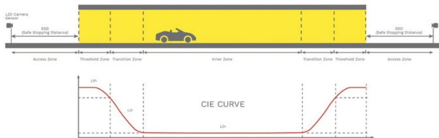
Figure 1: CIE Curve adjusted for bi-directional tunnel traffic.
