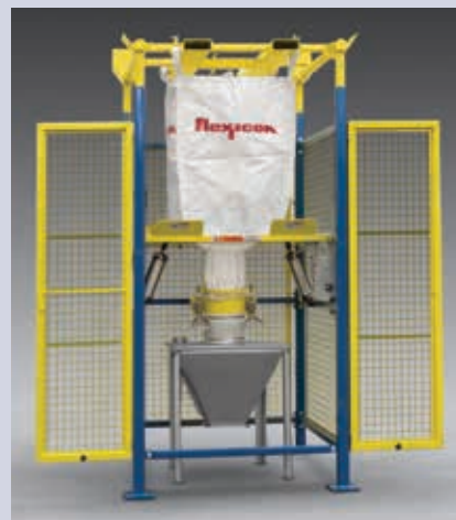
Steel safety enclosure of BULK-OUT™ Model BFF Bulk Bag Discharger ceases operation of moving parts when safety interlocked doors are open.
