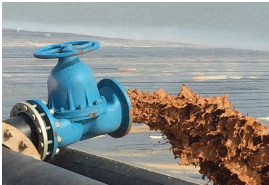
A locally manufactured KLEP BMG diaphragm valve discharging an abrasive slurry. BMG industrial slurry valves are designed to cope efficiently in harsh conditions and include butterfly, knife gate, diaphragm and pinch valves.
