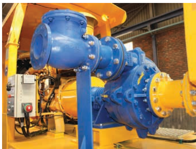
For dewatering, a diesel driven Warman DWU pump set on a trailer-mounted Multiflo unit can be used where access is impractical.
