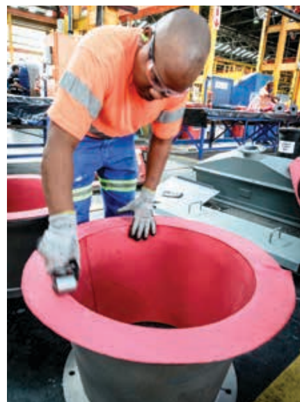
Weir Minerals' Linatex rubber lining delivers extended wear life, minimising plant downtime and can be installed on site.
