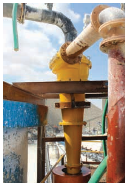
The Cavex hydrocyclone has a laminar spiral inlet that reduces turbulence resulting in greater efficiency and reduced wear life.
