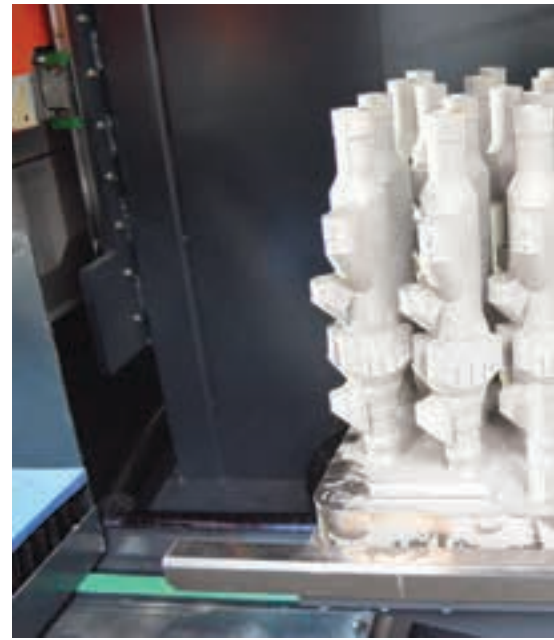
The titanium plates and components are then placed on the rotating clamping mechanism and attached using thick screws.
