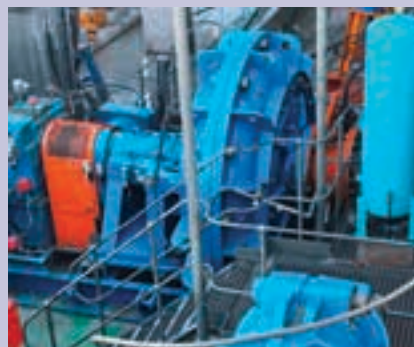
A Warman MCR 450 installed at Mogalakwena Mine. The MCR 450 runs at lower speeds resulting in lower wear rates on the parts.
