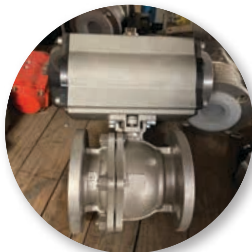
A pneumatically actuated ball valve used for automated process control.
