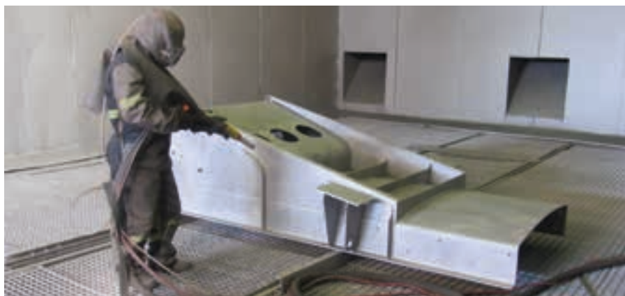
The shot blasting process ready to commence in Kwatani's purpose-built booth. Even the paint specifications come with certificates.
