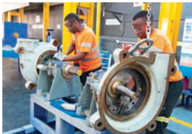
The local manufacturing process at Weir Minerals includes foundry and assembly capacity for producing slurry pumps.
