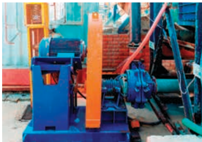
The new Warman WBH slurry pump with streamlined impeller inlet handles the most difficult slurries.
