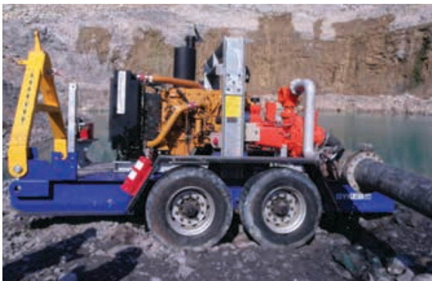
A Sykes Xtra High Head dewatering pump provided reliable dewatering to a mine in Lesotho.
