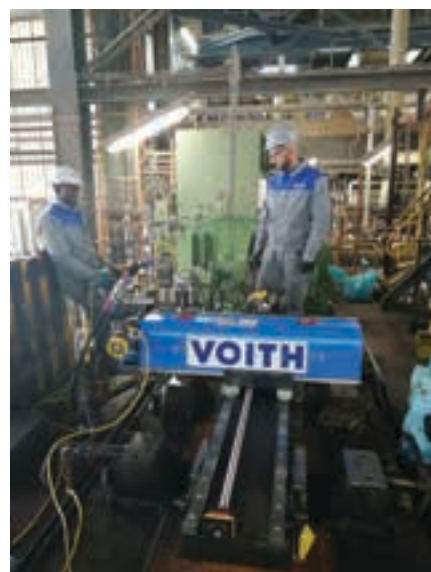
The linear mill is a bed-type milling machine for universal use in a fast and accurate way.
