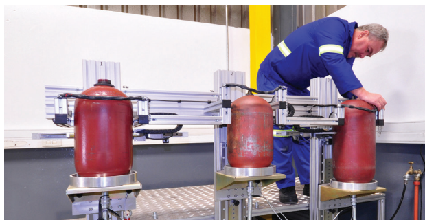
HFT conducts conformance testing on hydraulic accumulators, followed by refurbishments and recertifications
