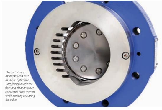
The flow is divided through the slots, which reduces cavitation because the stream bubbles occurring in the cartridge slot area are smaller because of the lower flow rate within each channel. Therefore, less energy is released when the stream bubbles implode. Furthermore, especially at small opening angles, TRI-SHARK valves are able to keep water jets concentric to the pipeline's centreline, thereby reducing their kinetic ener-
