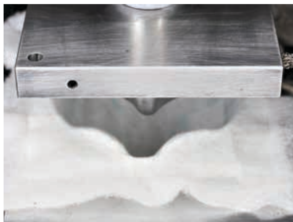
In order to start the production of the respiratory masks quickly, different companies supplied equipment for the deep-drawing process of the nonwovens.
