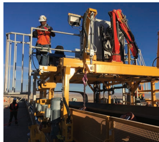
TAKRAF maintenance vehicle for safely lifting the belt and replacing the idlers.
