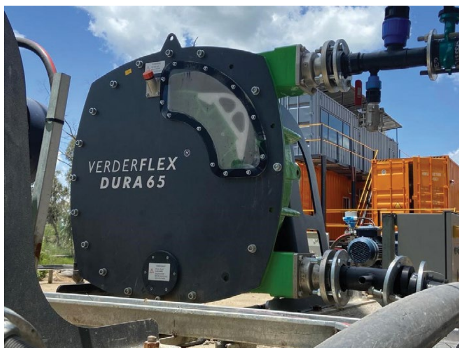
The completely redesigned Verderflex D65 – which has the same footprint and uses the same hose as its predecessor, the VF65 – offers a 20% better flow rate while also extending hose life by 20%.
