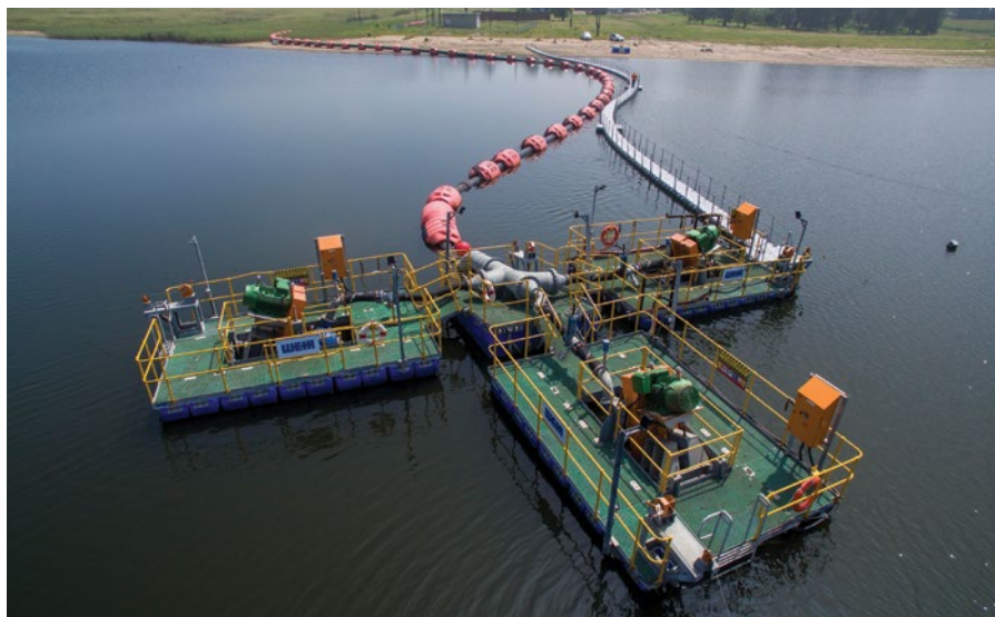
Weir Minerals offers engineered to order pontoon barges to suit its customers' dewatering requirements.
