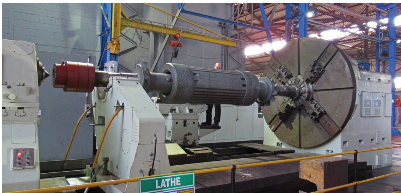
Sappi's 30 MW generator rotor undergoing dimensional checks in M&C's 140 t precision lathe that can handle 40 t work pieces that are 11 m long with a swing of 3.2 m.
