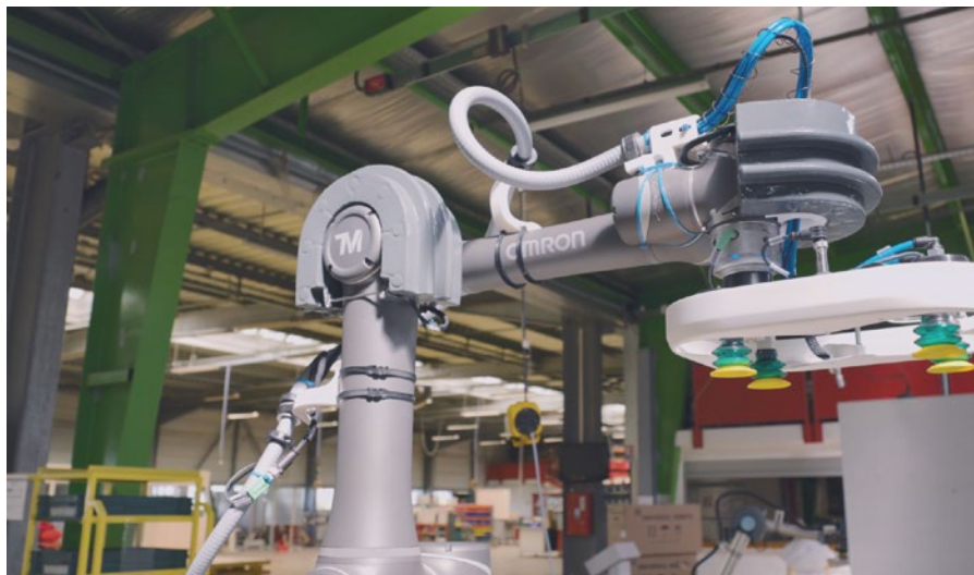
OMRON and FlexLink have designed a collaborative (cobot) palletiser for industrial applications.
