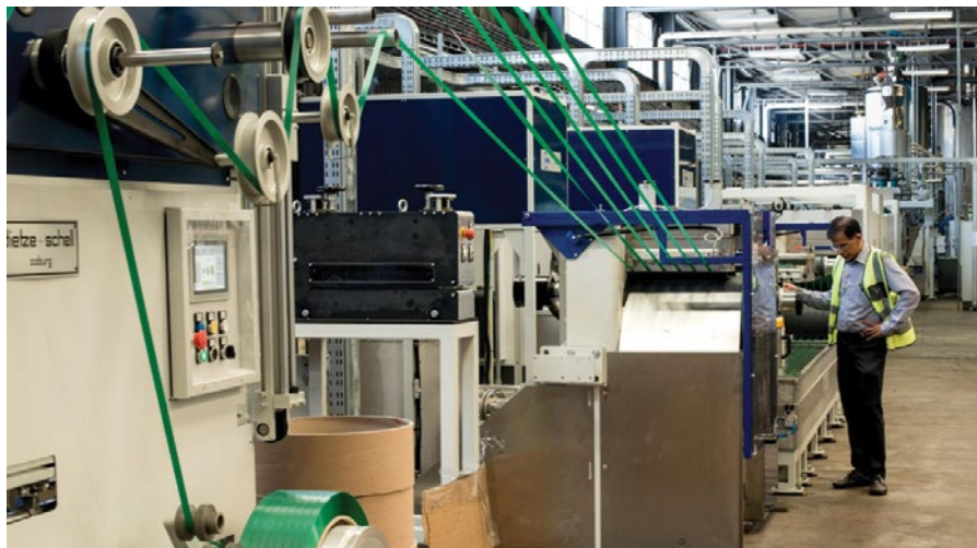
Dilip Jade, technical director of PET recycler, Extrupet, examines the company's new Sima line in Cape Town, which produces various types of recycled PET (rPET) strapping.
