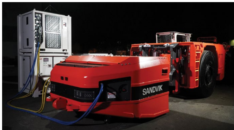
Equipped with patented AutoConnect and AutoSwap functions, Sandvik's LH518B underground BEV loader can change batteries on its own in just six minutes.
