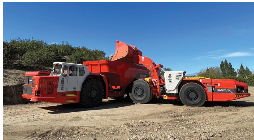
Equipped with patented AutoConnect and AutoSwap functions, Sandvik's LH518B underground BEV loader can change batteries on its own in just six minutes.
