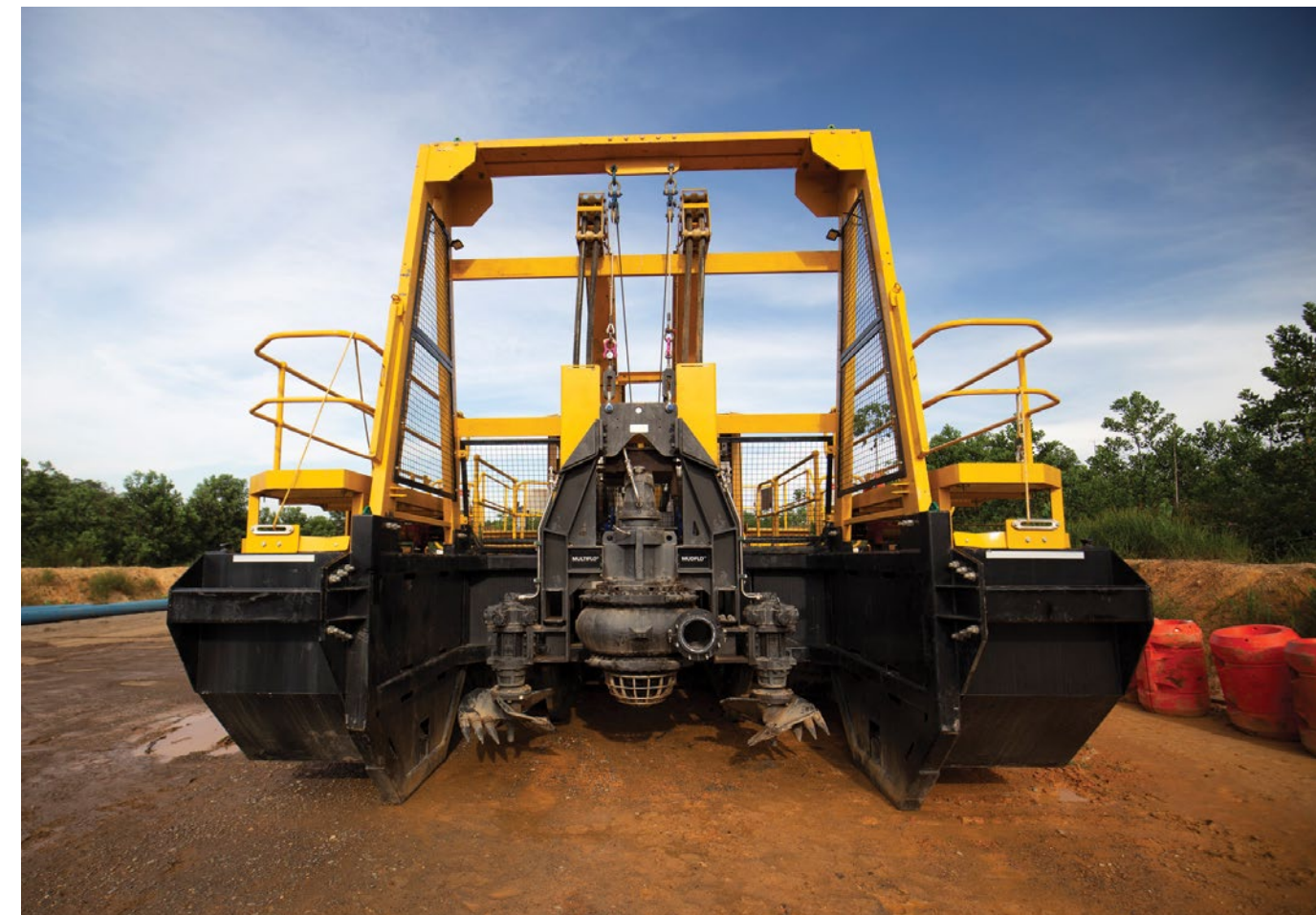
The Multiflo ® Mudflo ™ pump and dredge unit is paired with twin Multiflo ® CB33 hydraulic cutters with Weir ESCO ® excavation teeth.
