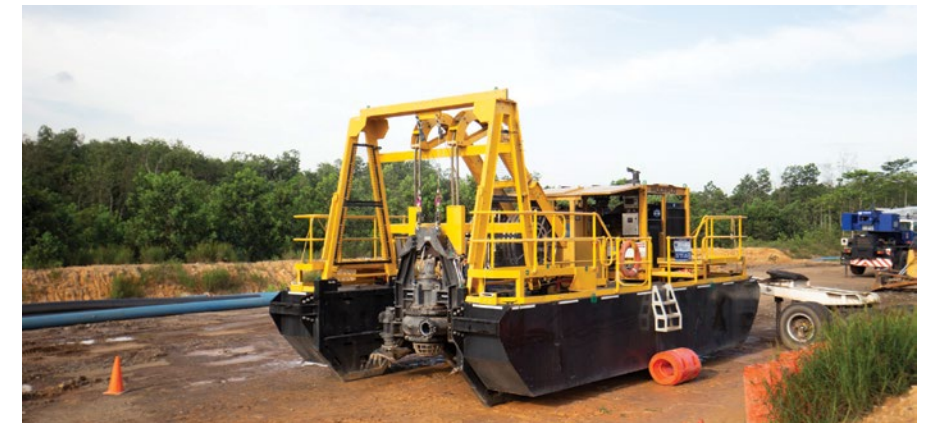
The Multiflo Mudflo pump was initially designed to address the constant challenge of mud caused by high rainfall, which was impeding production.
