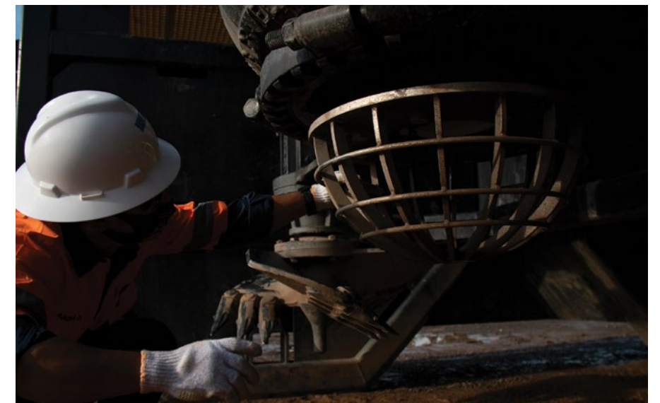
The Mudflo pump can be assembled onto the dredge unit on land, eliminating safety risks of assembling pumps over water.
