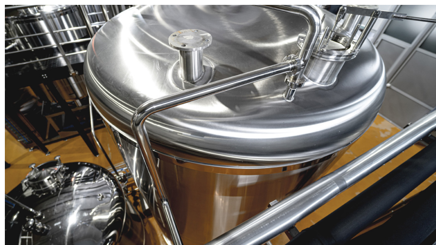
Cooker vessels in a food production facility will often use thermal energy such as steam as a key input in the beneficiation process.
