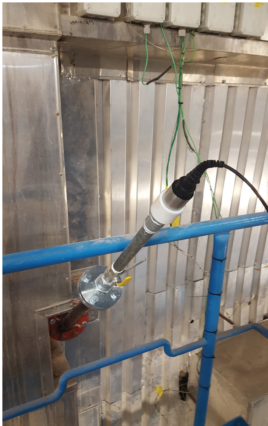
Acoustic microphones are used higher up, on the end of wave-guide air tubes that are bolted onto a flange on an entry point of the shell. An optional soot blower system can also be installed to keep acoustic waveguides clear of ash build-up.
