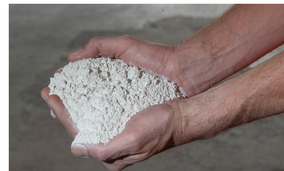
Left: LKAB's MicaFort product is used as a mineral filler for paint and coatings and other applications. Right: Final milled muscovite material has gone through size reduction, pneumatic conveying, drying and sieving steps.
