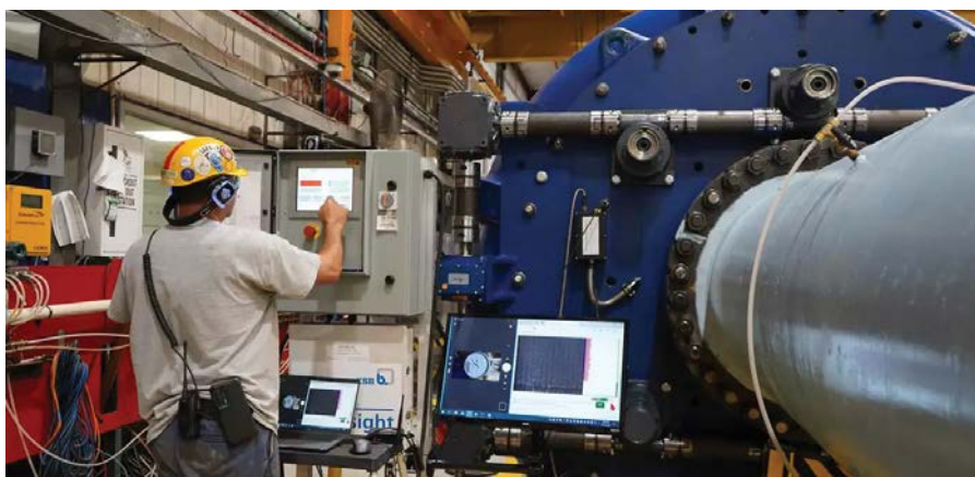
SLYsight is a slurry pump wear monitoring system that provides real-time data on pump wear.
