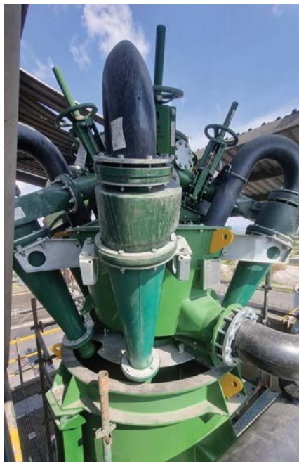
Left: An eight-way Multotec cluster of 250 mm cyclones at 10° with one barrel was selected for the desliming application. Right: Multotec's HX5 spiral with a pitch angle of 19° was found to achieve the best recovery and yields on the rougher stage.
