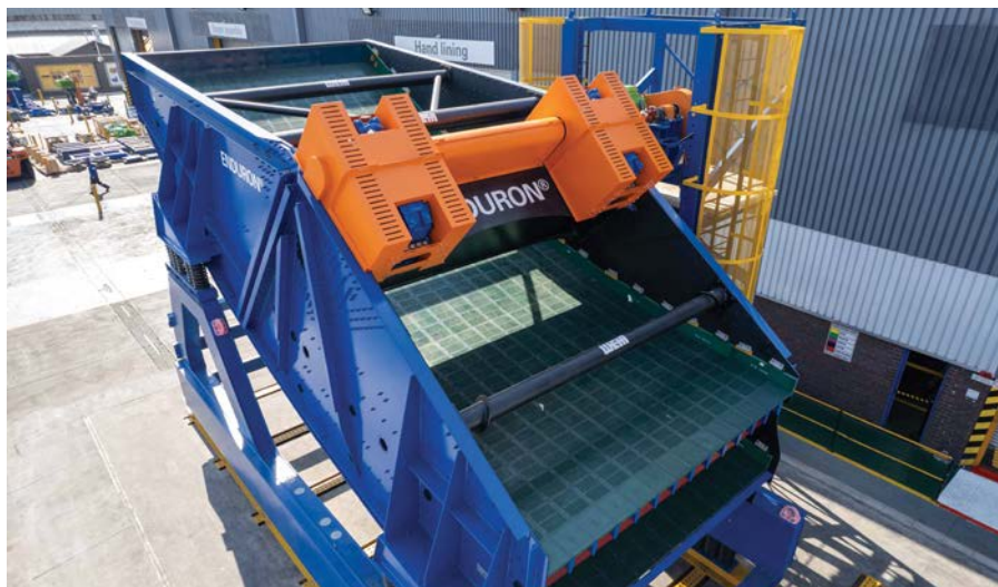
ENDURON Elite screens, weighing up to 50 tonnes, are driven by just two exciters thanks to their innovative, energy-efficient design.
