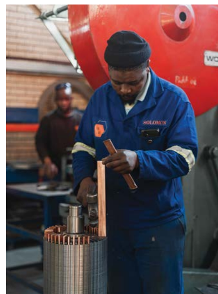
Barring the rotor of a squirrel cage induction motor with copper bars.
