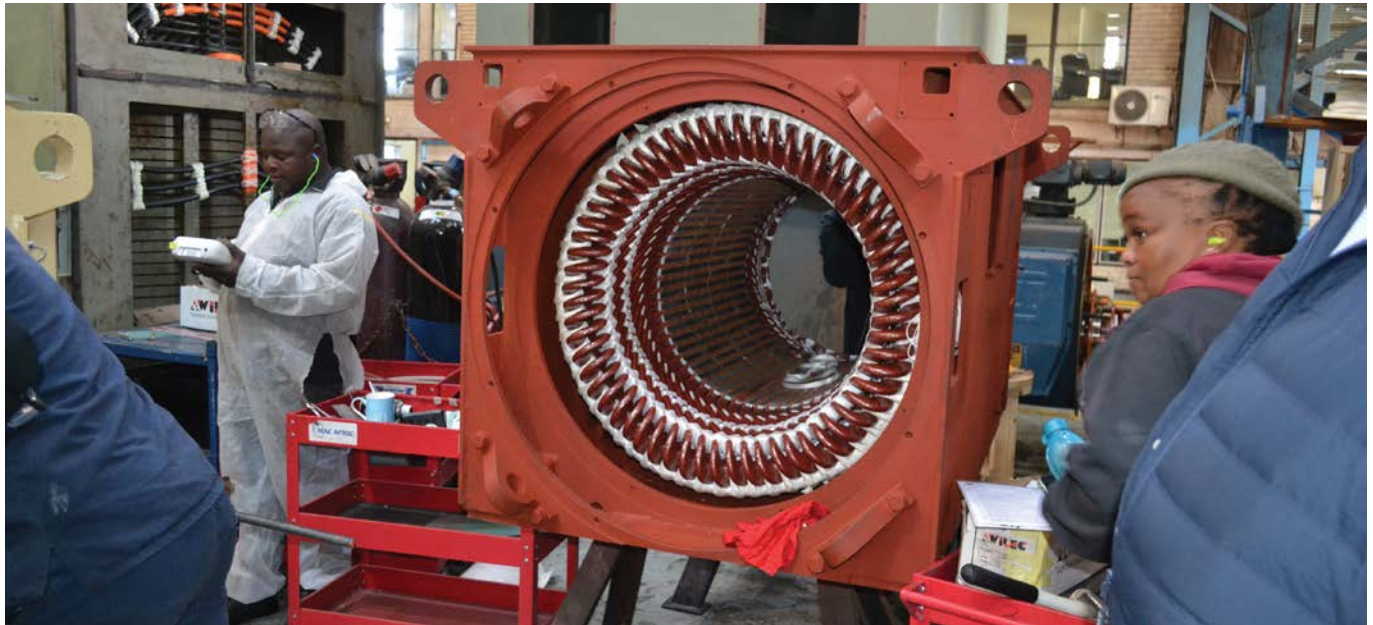
Form-wound copper stator coils are being installed for a motor at Marthinusen and Coutts' Cleveland facility.
