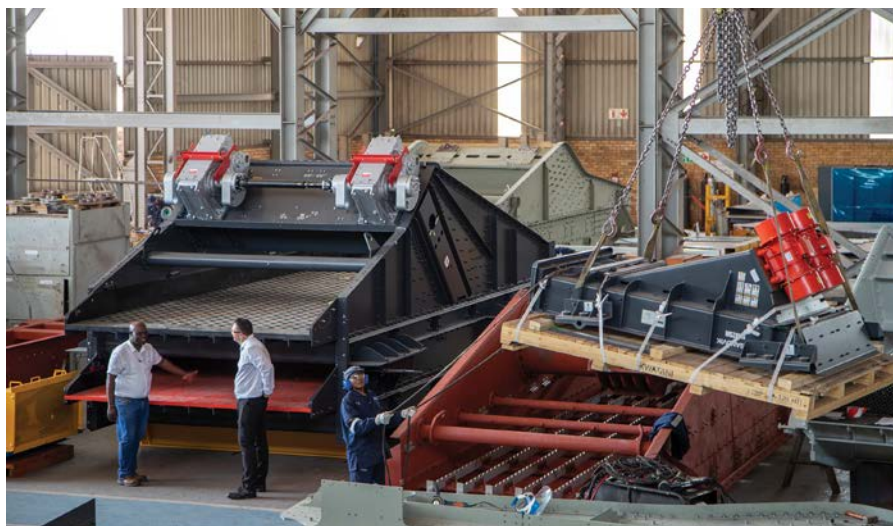
An SM Range horizontal double-deck exciter-driven screen with an S Range feeder being lifted by crane during on-site handling.
