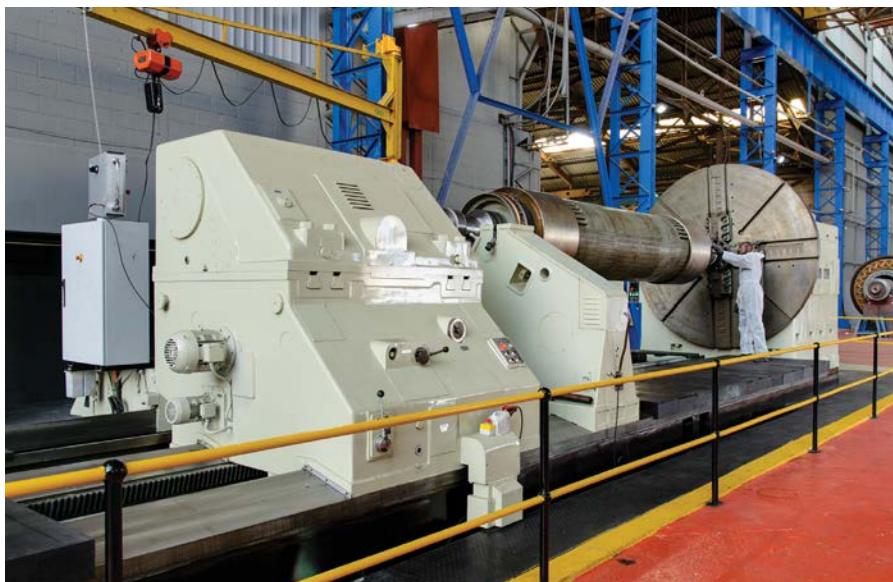
For very large machines, the Benoni facility includes a 140 t Wagner lathe that can accommodate a 40 t, 11 m workpiece with a swing of 3.2 m.
