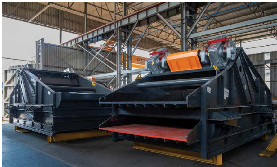
SRP's SM horizontal double deck exciter-driven screen is equipped with Sandvik screening media, ensuring consistent performance across tough applications.
