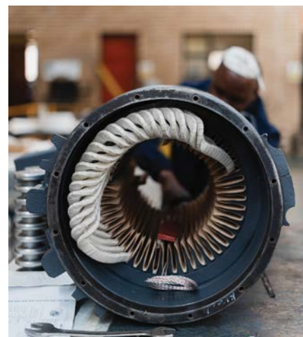
Winding of the stator coil of a flameproof water-cooled motor at Hexagon Electrical.
