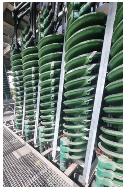
Left: An eight-way Multotec cluster of 250 mm cyclones at 10° with one barrel was selected for the desliming application. Right: Multotec's HX5 spiral with a pitch angle of 19° was found to achieve the best recovery and yields on the rougher stage.
