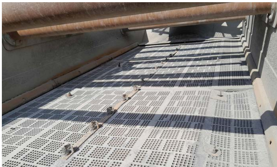
The conversion from woven wire mesh screening media to Multotec's side-tension polyurethane mats significantly reduced the customer's total cost of ownership.
