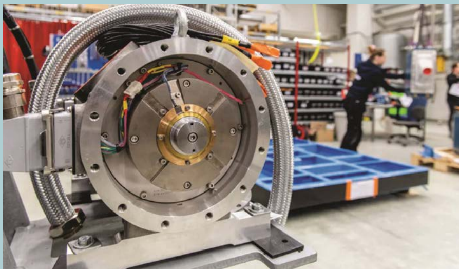
SKF magnetic bearing systems reduce energy use and eliminate oil-related pollution.
