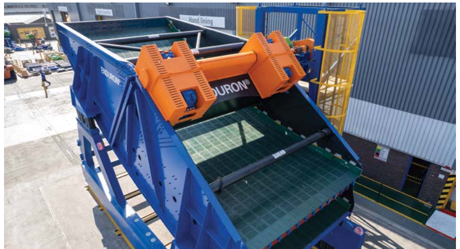
Weir's large ENDURON® Elite double-deck banana screens are being produced at the Alrode manufacturing facility in South Africa.
