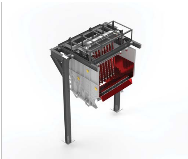
Left: A rendered image of Weba Chute Systems' custom-engineered jaw crusher feed chute, designed with swing doors to absorb impact and control ore flow, reducing wear from oversized run-of-mine material. Right: Rendered image of the apron feeder discharge chute, incorporating Weba Chute Systems' swing door design to manage high velocity flow, extend liner life and enhance reliability.
