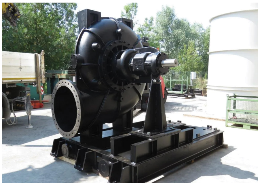
A SAER NCBK 800-670 pump purpose-designed to deliver 10 000 m 3 /h of water in an irrigation application for a rice paddy.
