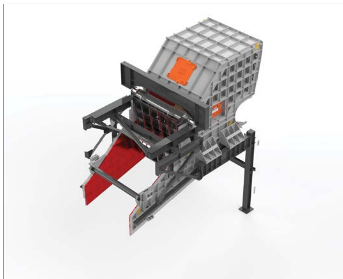
Left: A rendered image of Weba Chute Systems' custom-engineered jaw crusher feed chute, designed with swing doors to absorb impact and control ore flow, reducing wear from oversized run-of-mine material. Right: Rendered image of the apron feeder discharge chute, incorporating Weba Chute Systems' swing door design to manage high velocity flow, extend liner life and enhance reliability.
