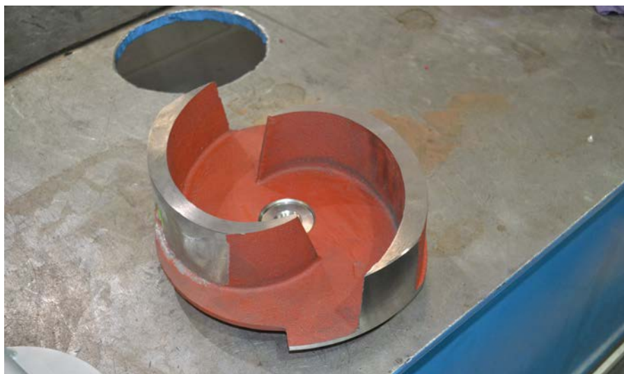
The market-leading impeller design enables the Imvubu pump to pass a larger solid (77.3 mm) than any of its competitors in the wastewater sector.
