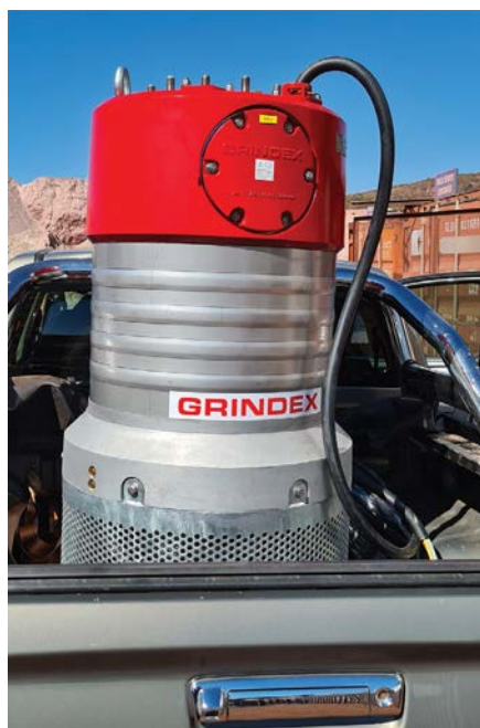
The Grindex H series is capable of pumping water to impressive heights of up to 180 m from deep-level mines.
