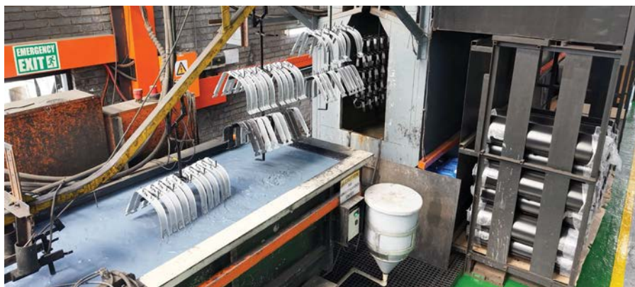
The 'closed loop' conveyor system guarantees repeatability in key areas, from ensuring that no process is omitted to achieving contact time repeatability, which is fundamental to quality and optimising repeatable coverage.
