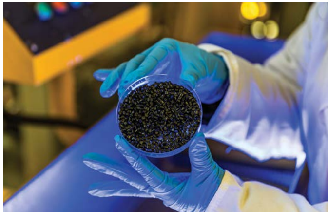
Left: CSIR-developed advanced nano-reinforced polymer composite pellets. Right: The advanced nano-reinforced polymer composite developed and produced for 3-D printing by Filament Factory.
