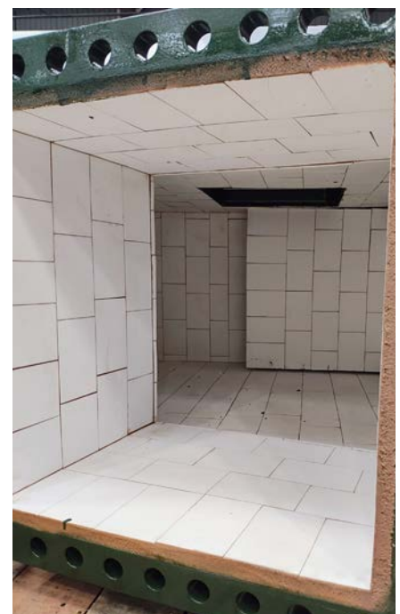
Left: Multotec lined 23 chutes in Brazil and will redesign and line new chutes using insights from current wear patterns to improve wear resistance. Right: A lithium producer in Brazil upgraded its chutes from rubber lining to Multotec's custom ceramic lining, achieving a significant improvement in wear life.
