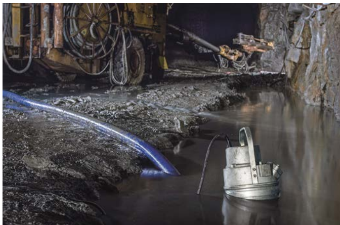
Left: Integrated Pump Technology's Grindex Mega INOX pump in action at a Zambian mining site, delivering reliable dewatering from the tailings dam to the process plant. Right: The 85 kW Grindex Mega INOX pump has operated continuously for nearly a year, meeting the mine's high head and flow requirements with ease.
