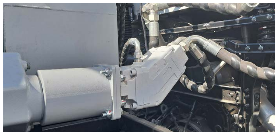
With fewer moving parts exposed to environmental stress factors, hydraulic drives are less vulnerable to the mechanical failures that often plague belt-driven setups.
