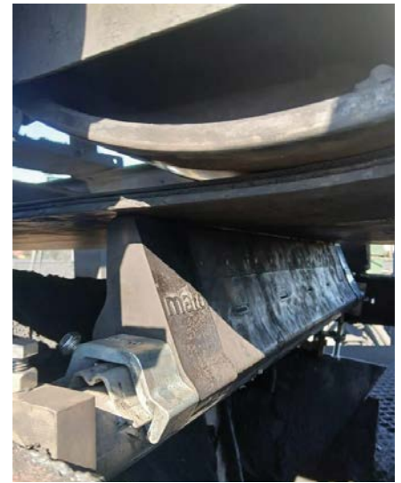
Left: The first and most significant advantage of Mato's diagonal tail pulley cleaner is that it is easy to install. Right: MATO Unique (MU) secondary cleaners are located beneath the belt, behind the primary, to remove stubborn material from the underside of the belt.
