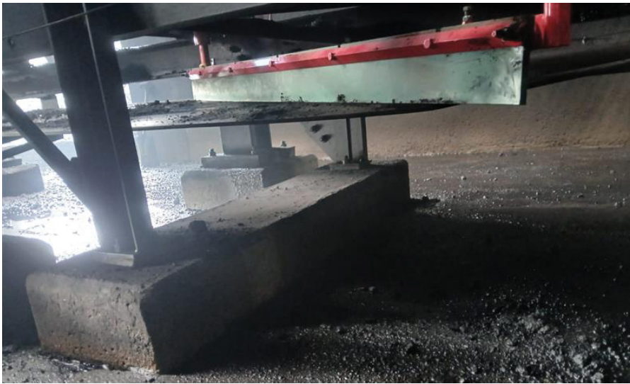
Left: The first and most significant advantage of Mato's diagonal tail pulley cleaner is that it is easy to install. Right: MATO Unique (MU) secondary cleaners are located beneath the belt, behind the primary, to remove stubborn material from the underside of the belt.
