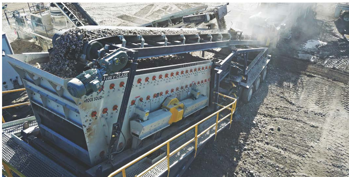
Integrating eccentric screening technology, state-of-the-art screen media, and diagnostic tools can prevent blinding, pegging, carryover, and contamination, thereby improving screening performance, productivity, and profitability.
