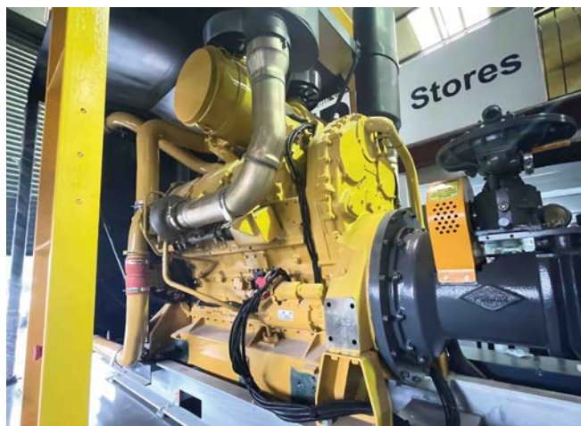
Left: The PAC SH high-head pump is built to handle high concentrations of solids and abrasive materials, making it well-suited to demanding site conditions. Right: The PAC SH pump’s lower fuel consumption and longer service intervals help reduce overall operating costs.
