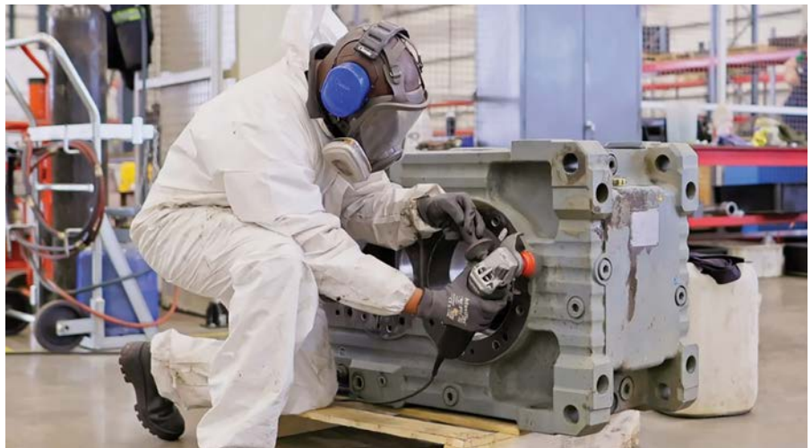
Dedicated assembly lines at the new Service Centre will enable SEW-EURODRIVE to deliver fully remanufactured gearboxes in as-new condition, with improved turnaround times.
