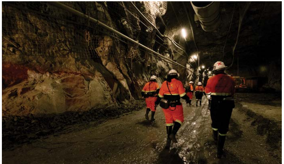
Venetia is using a progressive sublevel caving operation, where multiple drives will be developed, but only a few will be mined at any one time.
