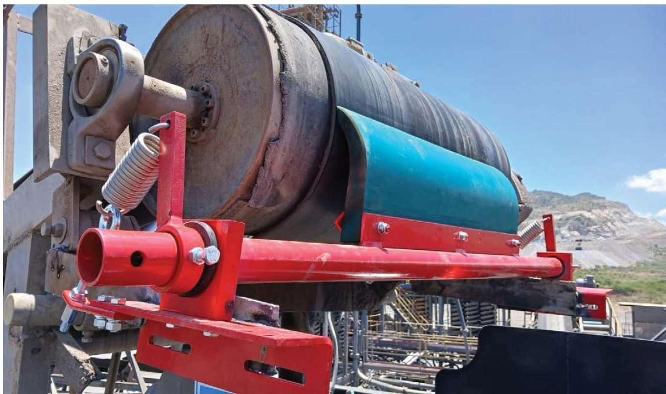
The primary cleaner on a conveyor belt sits on the drive pulley beneath the discharge stream and handles about 90% of carry-back material.
