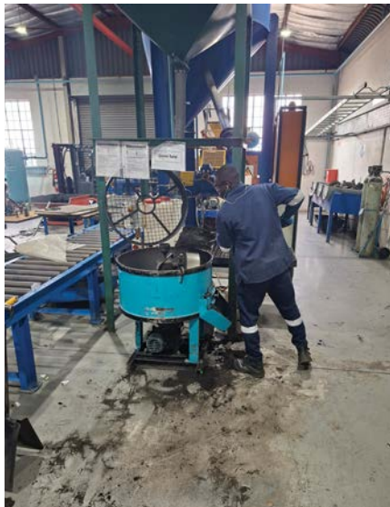
Left: The GFTC's pattern-making shop: The college is introducing digitalisation, with employees moving from manual design to computer-aided design. Middle: A trainee doing sand preparation at the GFTC's foundry using a green sand mixer. Right: A motorised sieve shaker for sand testing and quality control.
