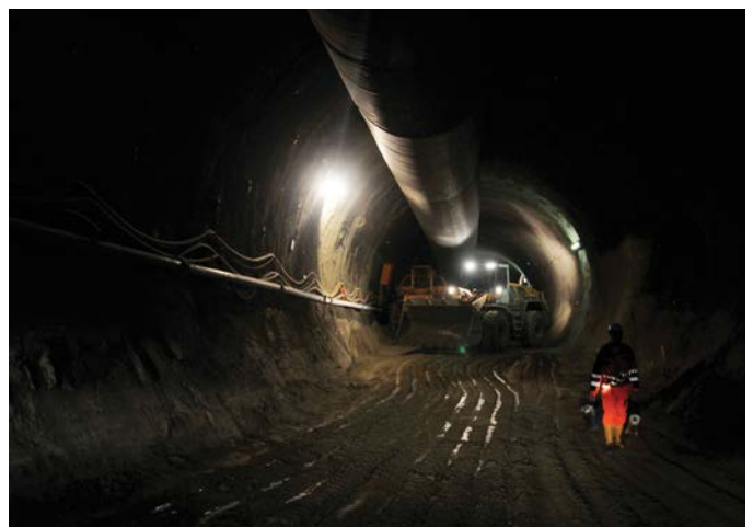
Left: Contaminants released into the mine ventilation system must be diluted and exhausted from the mine, and the only way to do that is to increase ventilation levels. Right: While EVs can reduce refrigeration demand compared with diesel fleets, the reduction is constrained by minimum air-velocity requirements, and the overall benefit depends strongly on the mining method.
