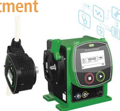
The peristaltic Verderflex Ds500 metering and dosing pump contains the pumped chemical within the tube element, ensuring it never comes into contact with the pump's mechanical components.
