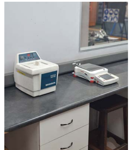
Some of the GFTC's precision laboratory equipment: a Branson 1510 ultrasonic cleaner used to separate clay from sand grains in a sample, and an Ohaus Explorer precision balance for achieving an exact chemical composition of a melt.
