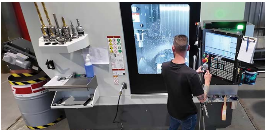
Werner Pumps' new 5-axis CNC machine enables highly precise machining of complex components from a single block of material in a single, integrated process.
