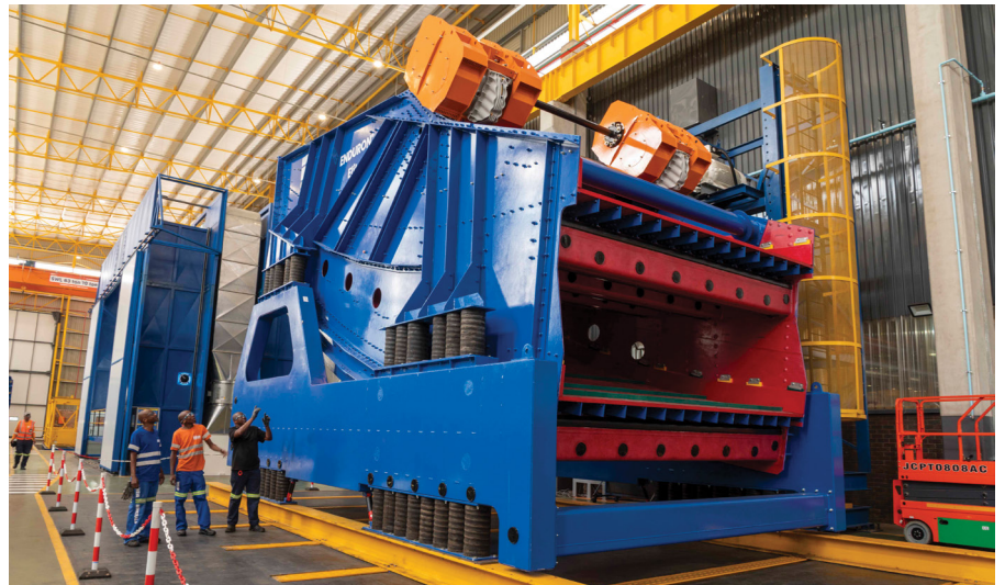
The new heavy bay screen manufacturing facility at Weir Alrode is now producing ENDURON Elite double-deck banana screens for the Reko Diq order.
