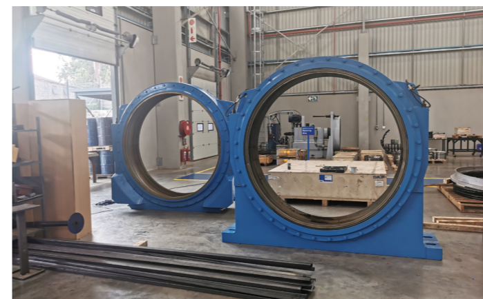
Left: Locally manufactured trunnion housing assemblies. One housing has been remanufactured, and the lead time has been reduced from 10 weeks for new production to 3 weeks for remanufacturing. Right: A set of SKF plummer block housings for mill pinions that were custom-designed and manufactured in South Africa.
