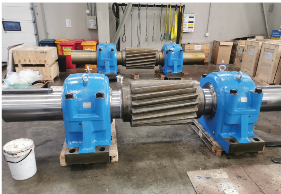
For horizontal grinding mills, SKF South Africa can custom-engineer and locally manufacture mill pinion housing assemblies.
