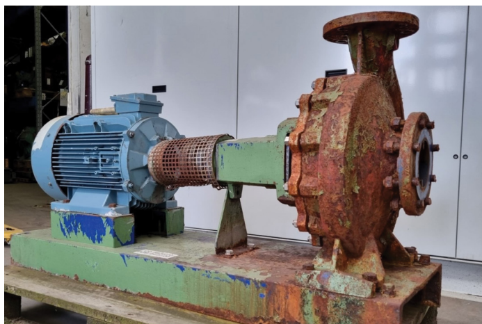
Left: KSB ETAnorm irrigation pumpsets, if well maintained, will still be operating after 20 years of irrigating crops. Right: A critical water pump station in Freestate, where two FBL 500-400 Double Suction Split Casing Pumps have been in operation since 1967. They were built in South Africa and regularly maintained.
