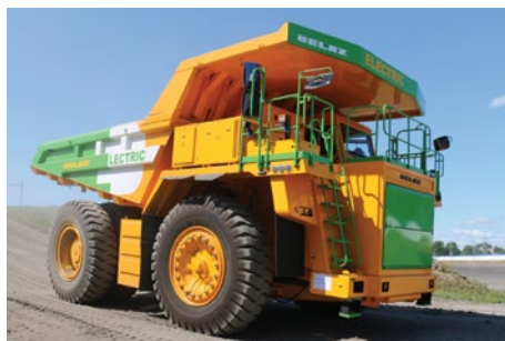
This is a completely new type of mining haul truck, featuring batteries instead of a diesel engine.
