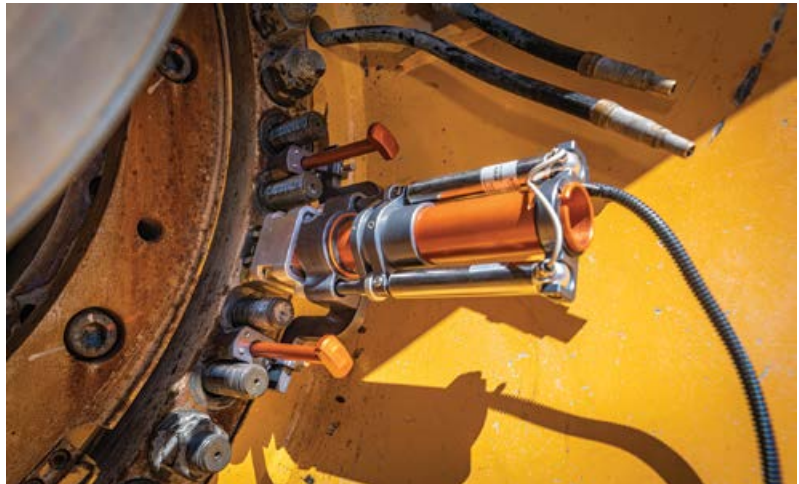
Above and left: Kal Tire's Kal Clamp offers a step-change in the tyre removal process.
