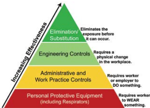
Hierarchy of controls - remote monitoring with N2 delivers optimum control of risk by eliminating exposure before it can occur.
