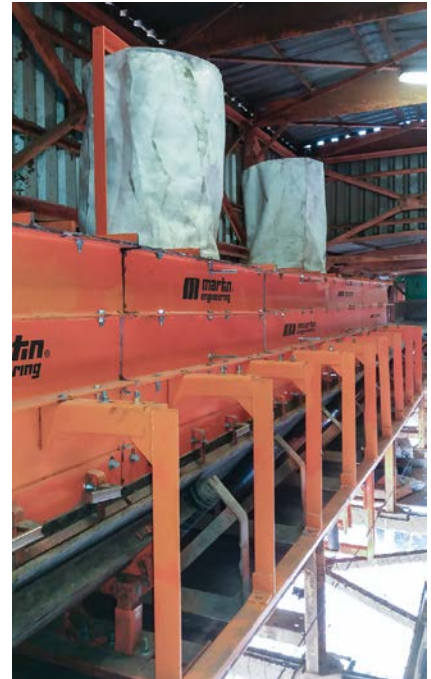
The new loading zone featured a sealing system that mitigated spillage and dust supported by dust bags.
