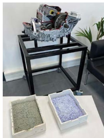
Magnet REO product laid out in Ionic Technologies' showroom in front of a permanent magnet synchronous motor (PMSM), showing >99.5% grade Nd203 product on right.
