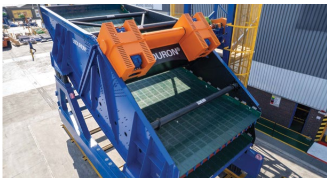
ENDURON Elite screens, weighing up to 50 tonnes, are driven by just two exciters thanks to their innovative, energy-efficient design.
