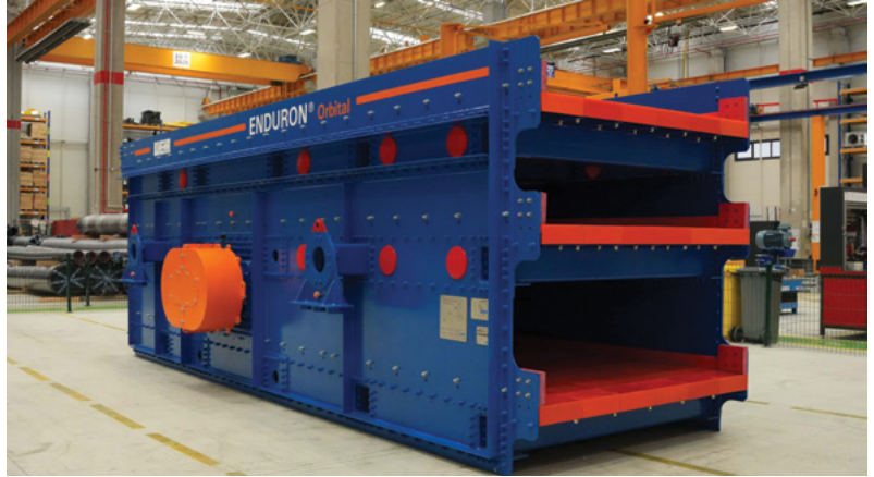
Weir recently launched the ENDURON® Orbital circular motion screens for smaller tonnage mining in aggregate and sand applications.
