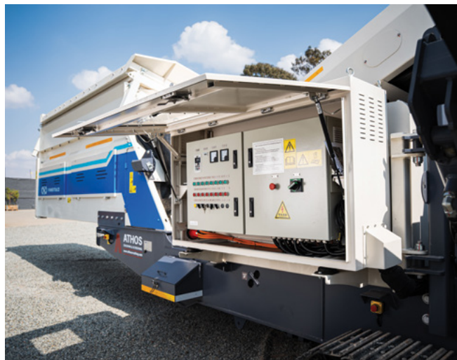
The Powertrack PT Pro ST-08E triple-deck screen brings high-capacity material separation with the advantages of a fully electric drive.
