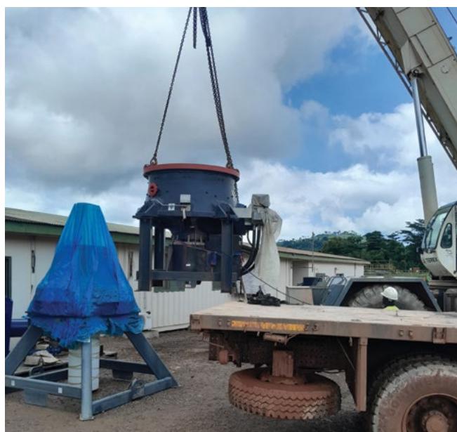
Components for the new Sandvik CH851i cone crusher supplied by Sandvik Rock Processing being offloaded on site at a gold mine in Ghana.
