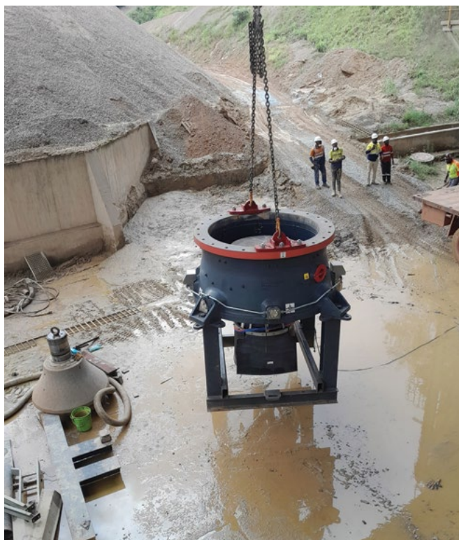
The bottom shell of the new Sandvik CH851i cone crusher supplied by Sandvik Rock Processing being offloaded from its stand and lowered to the ground.
