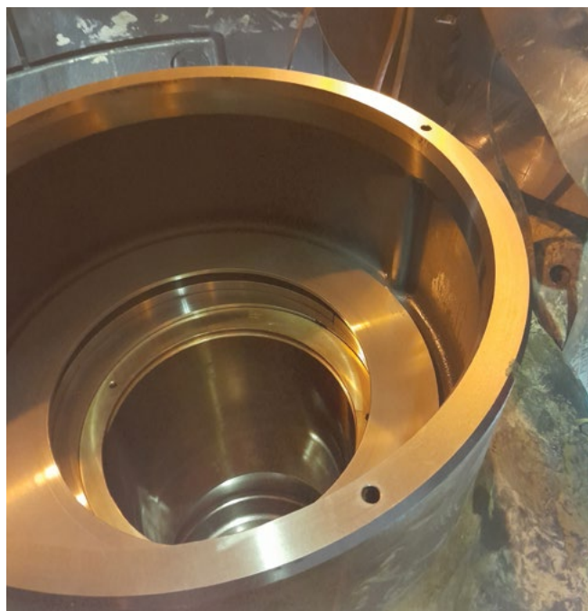
A view of the eccentric bush within the Sandvik CH865i cone crusher assembly.
