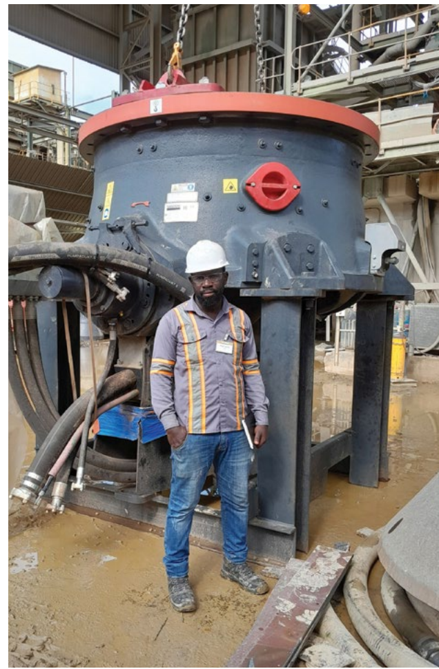
The bottom shell of the new Sandvik CH865i cone crusher supplied by Sandvik Rock Processing positioned on the ground in preparation for lifting into place.
