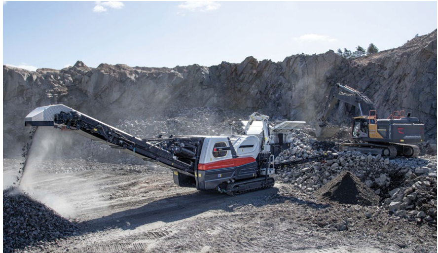
The extended discharge conveyor offers three operating positions, improving stockpiling flexibility and maintenance access.
