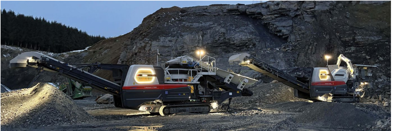
The advanced diesel-electric drive system on the Metso Lokotrack LT400J enables lower fuel consumption and reduced operating costs.
