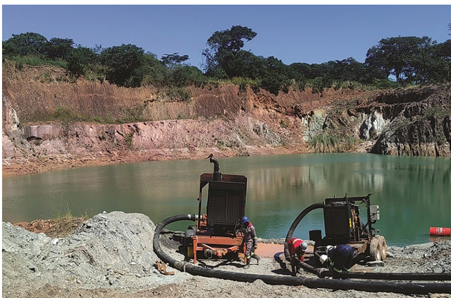
With proven durability and self-priming design, Godwin diesel-driven pumps deliver versatile dewatering solutions that reduce downtime.
