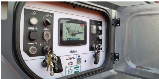
The control panel of the Metso Lokotrack LT400J integrates advanced IC process automation, enabling operators to monitor key parameters and adjust crusher settings for consistent, efficient production.
