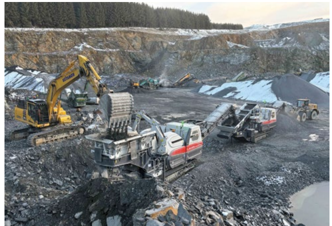
The extended discharge conveyor offers three operating positions, improving stockpiling flexibility and maintenance access.
