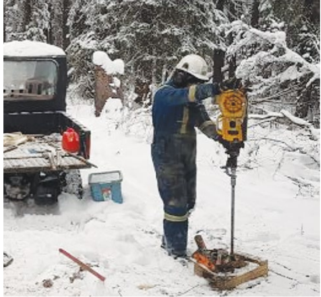
Fulcrum Metals undertaking auger drilling at Teck Hughes.
