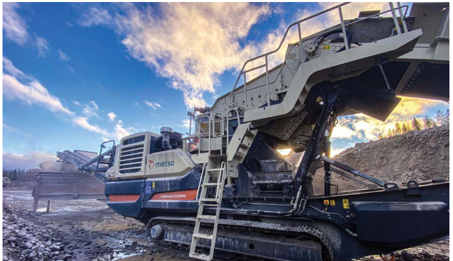
The LT200HPX is equipped with a two deck pre-screen and wide feeding and production conveyors to significantly increase production capacity.
