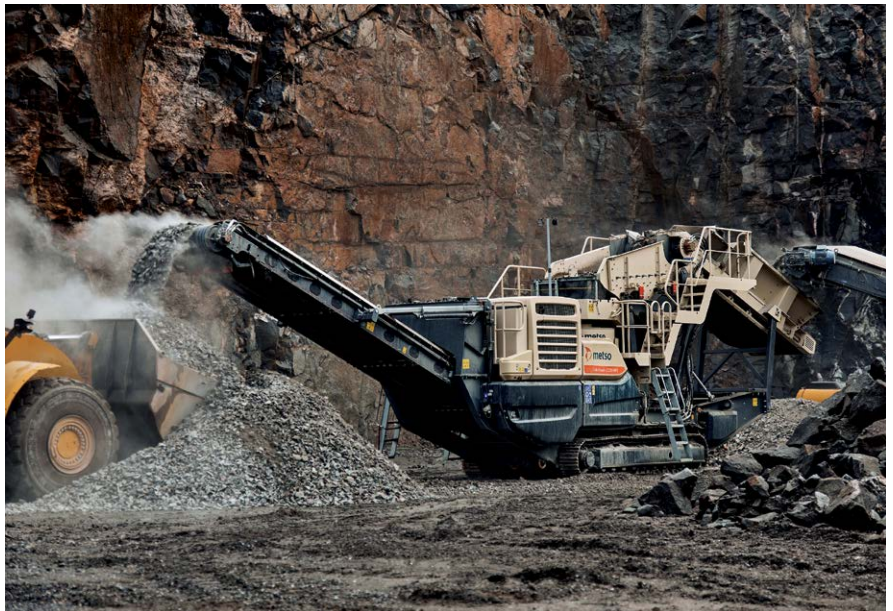
LT200HPX™ mobile cone crusher is especially suitable for a secondary or tertiary crusher in a 2 or 3 stage crushing process.
