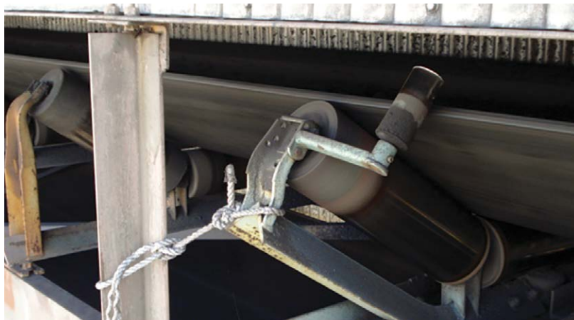
A tracking idler tied off to limit its travel.
