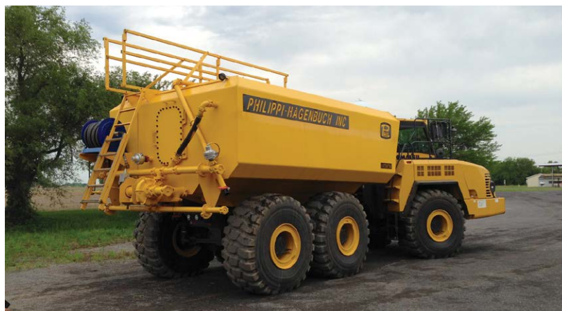
PHIL water tanks have baffling from floor to ceiling, as well as along the complete length and width of the tank, resulting in full compartmentalisation of the water and less surging.
