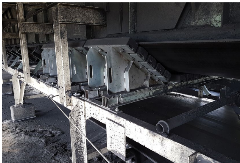
A Tru-Trac impact bed absorbing impact at a transfer point.
