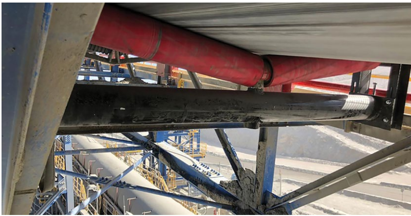
A Tru-Trac V-Return Tracker keeping the conveyor centred in a dry cargo handling application.
