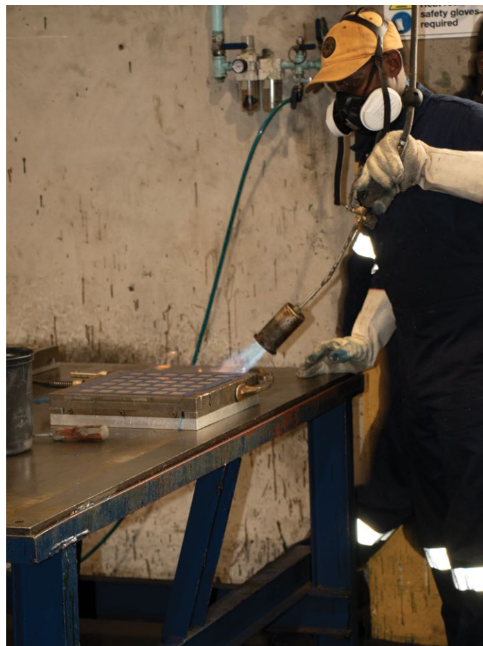
Flaming to remove any moisture after polyurethane casting into moulds.
