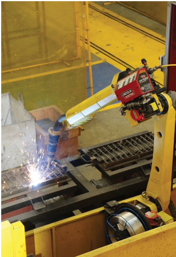
Robotic welding of screen panel inserts for optimised productivity.
