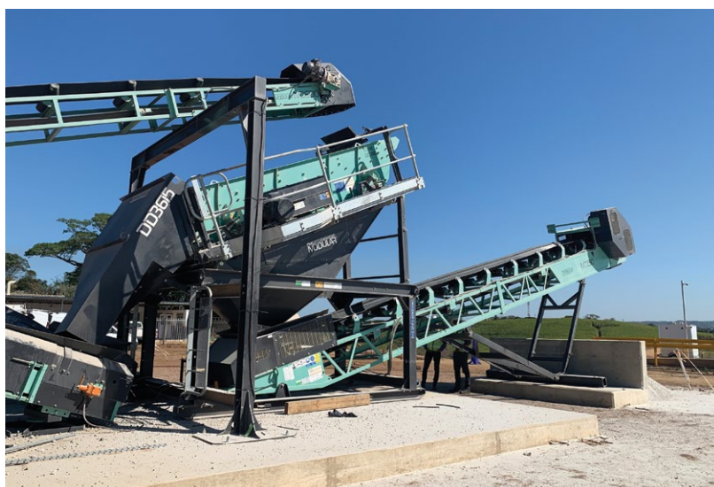
The Pilot Modular DD3615 Screen's double deck screen is 3,6 m x 1,5 m.
