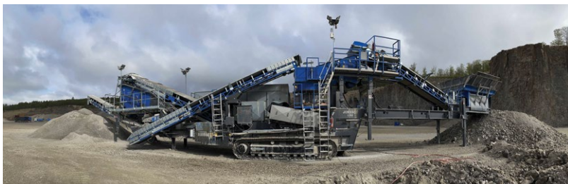
The L 550 is one of the largest mobile cone crushers on tracks and a mobile secondary crushing unit.
