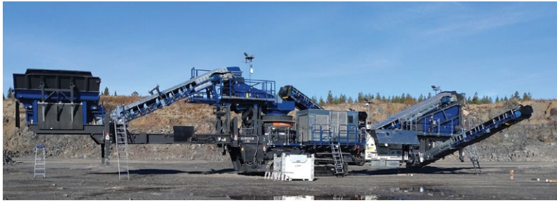
The L 400 is a mobile secondary crushing unit, as well as an adaptable third stage.
