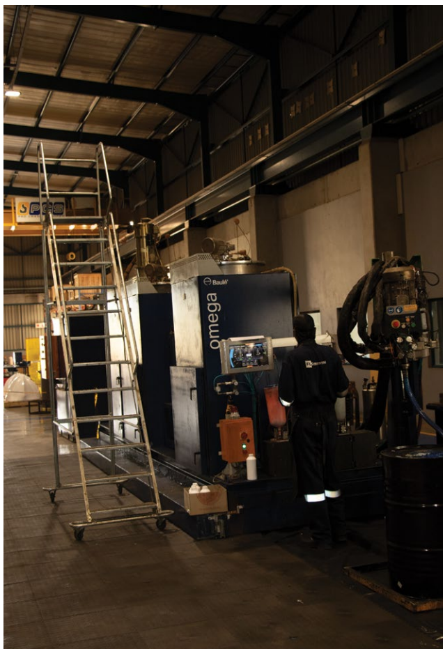
Latest generation high capacity polyurethane casting machine.
