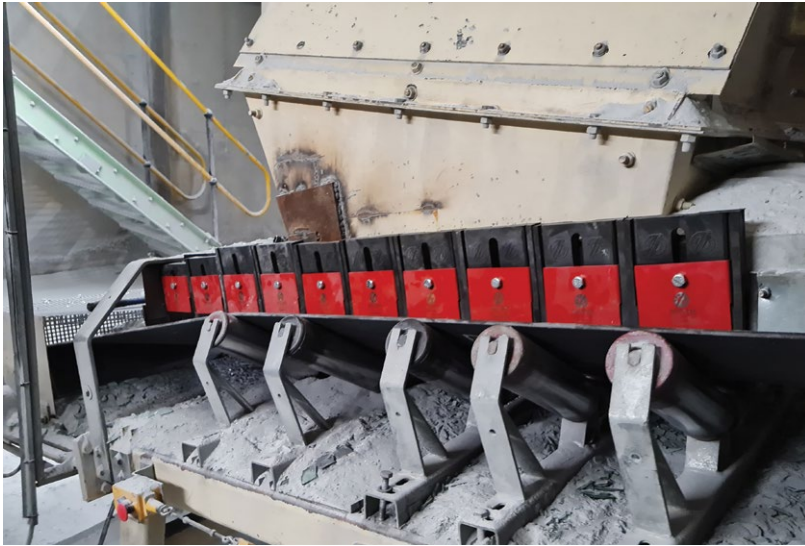
Use of Tru-Trac I-Lock skirting will prevent loss of material on conveyor handling equipment.
