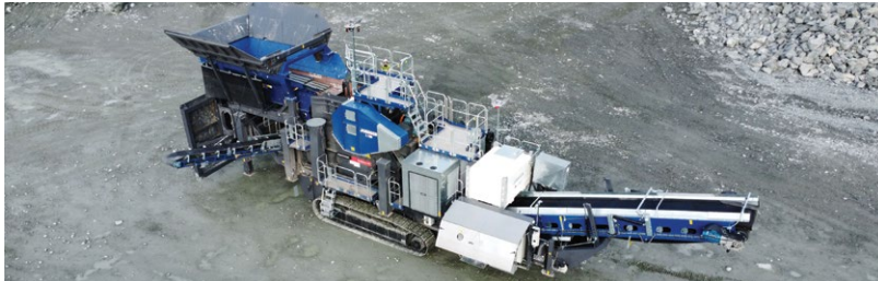
The L 150 mobile jaw crusher is powered by a 400kVA generator set or via mains operation and is equipped with a Nordberg C150 jaw crusher.
