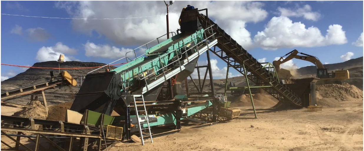
It is the fact that the two boxes can be run independently on their own drives that truly makes the Pilot Modular DD7215 semi-mobile screen come into its own
