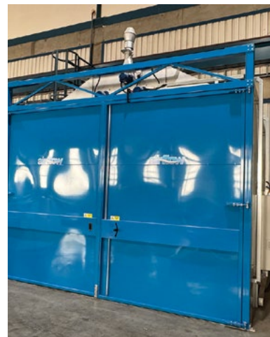
A new preheat and post-curing oven has been installed at FLS to boost production efficiency and ensure consistent high-quality curing of polyurethane products.
