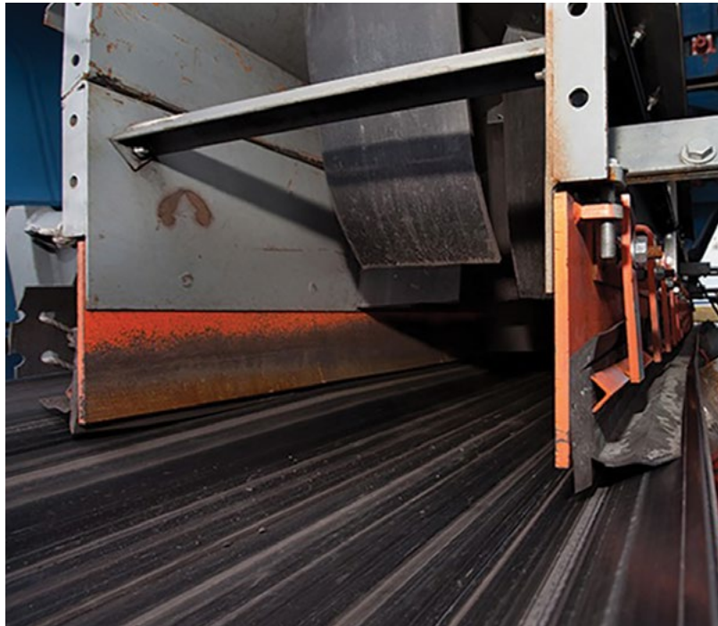
A properly structured enclosure is slightly elevated, with dust curtains, an external wearliner, and adequate skirting.
