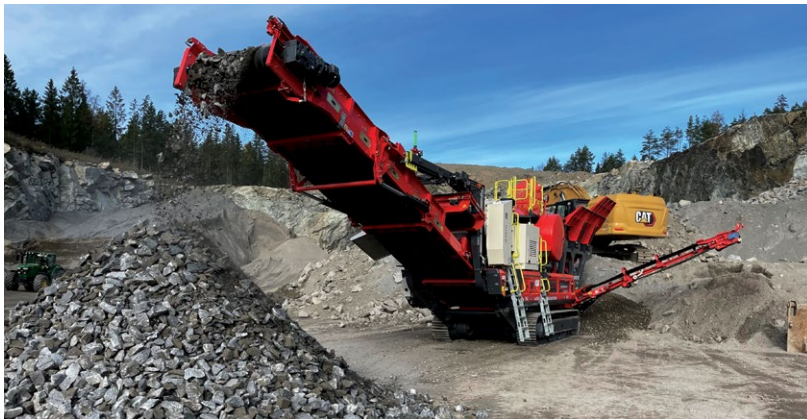
Designed for lower emissions and operating costs, the Sandvik UJ443E can run directly from the electrical grid or switch to diesel or renewable HVO fuels when required.
