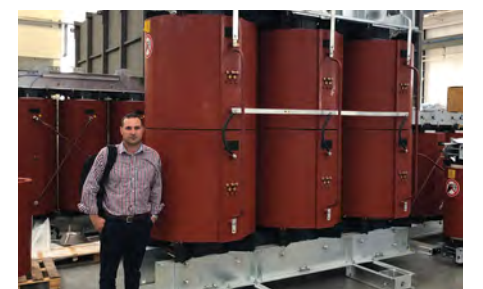
David Claassen, managing director of Trafo Power Solutions, in front of a 10 MVA cast resin transformer ideal for high power demands.
