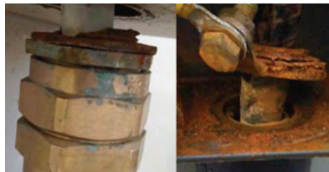
De-zincification results in glands becoming brittle and breaking. They can become detached, affecting the earth continuity and causing the installation to fail completely.
