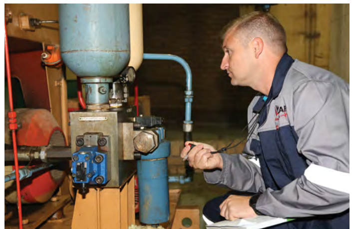
WearCheck advanced technical compliance technician, Joe Kies, measures the charging time of the hydraulic system for a winder.
