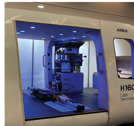
Airbus H160 rescue helicopter cabin mock-up with LINDO aBL multi-function lights in disinfection mode.
